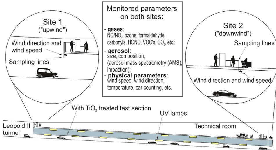
Fig. 2. Schematic representation of the test sites in the Leopold II tunnel during the PhotoPAQ campaigns.
