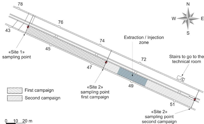
Fig. 3. Plan view of the tunnel test section for the first and second tunnel campaign.
