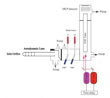
**Fig. 1.** Schematic diagram of Laser 2 steps Desorption Ionization Mass Spectrometry (L2DI-MS) technique (figure updated from Gaie-levrel et al., 2012).
